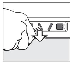
■ Insert a screwdriver into the notch of the left opening and pull downwards. The door will now open.
